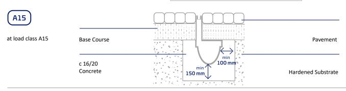
Load classes according to PN-EN 1433:2005 correspond to usage conditions from which proper type of grating and cover should be chosen.
